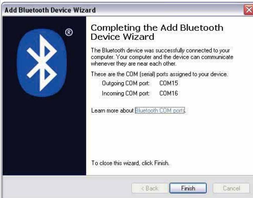
The Outgoing COM port will be the COM port which we have to use for further communication to that device. Click the Finish-Button.
