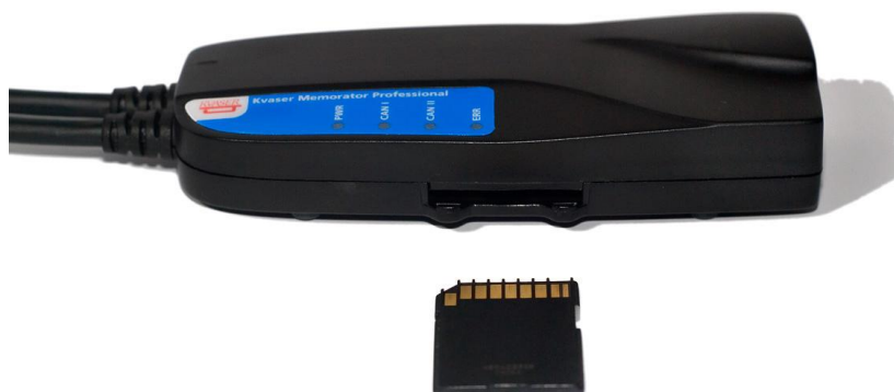
Figure 4: How to insert a memory card.
