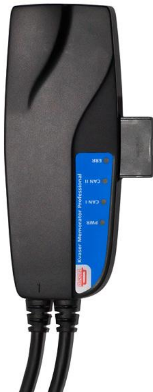
Figure 3: The CAN channels on Kvaser Memorator Professional.
