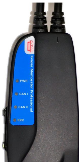
Figure 5. LEDs on the Kvaser Memorator Professional.
