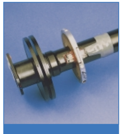
Torque data collection with temperature measurement on gas turbine output shaft
