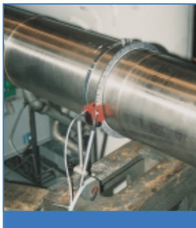
Shear and torque measurement on drive shaft
