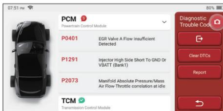
The system with DTC will be displayed on the screen in red font, and the specific number of DTC will be shown. A DTC-free system will be displayed as "OK".
